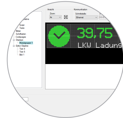
Configuration software for truck scale display
